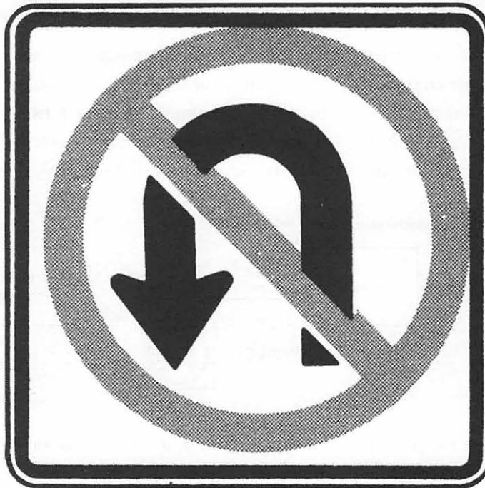
2-6: "NO U-TURN" sign
