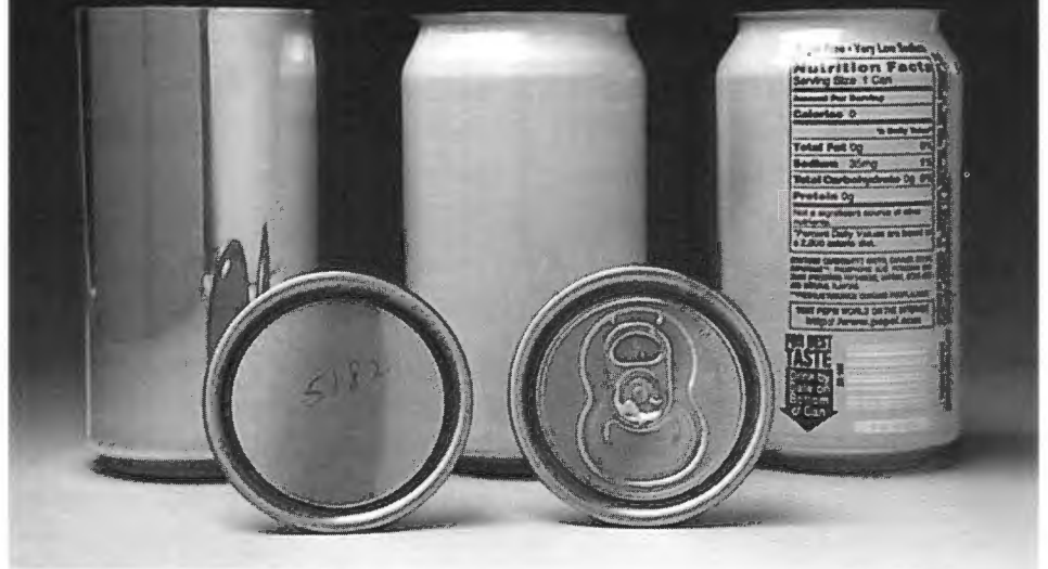
A-13: Aluminum can showing domed bottom
