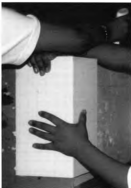
4-45: Adding cardboard flap to strengthen back-to-side joint
