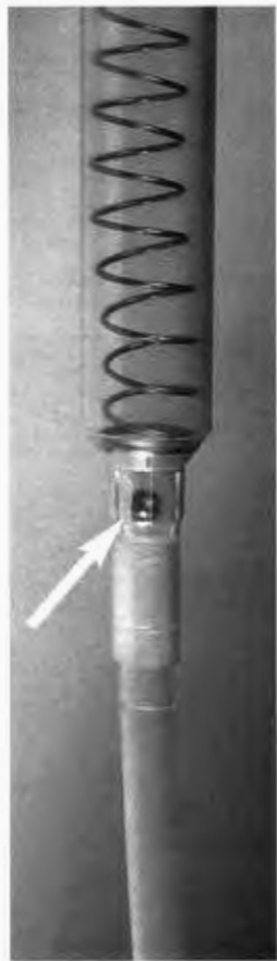
A-21: Detail of pump dispenser, showing ball valve
