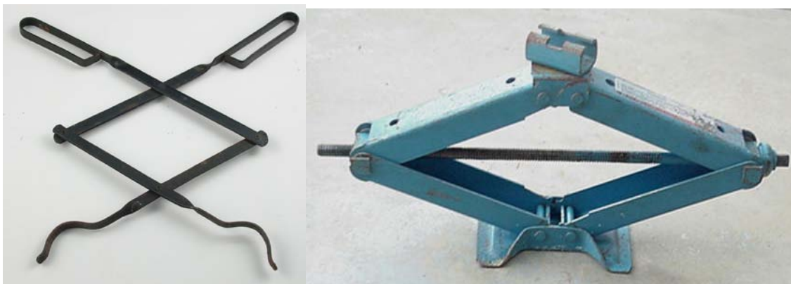
Figure 1: Four-bar linkages: fireplace tongs (left); scissor jack (right)
